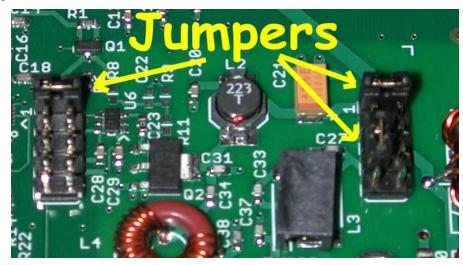
On P4, pins 1 and 2 need a jumper. (Input clock) On P3, pins 1 and 2 need a jumper. (+12V power) On P3, pins 5 and 7 need a jumper. (Antenna out)
